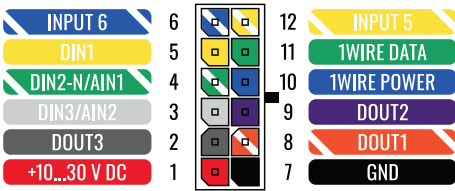
Secure S5/S7 4G 2x6 socket pinout
